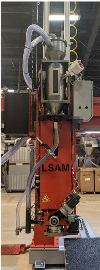
The 40-60mm print heads used on our flagship machines weigh well over two tons and require a significant machine structure and powerful servo drives to achieve optimum performance. To accommodate the request for a lower cost system, Thermwood refined and updated a 30mm print head design, initially developed during their print technology development.
