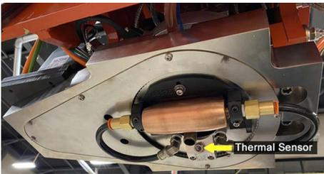
Thermwood's new Thermal Sensor Layer Automation System is also available on the LSAM Additive Printers. This is an exciting
