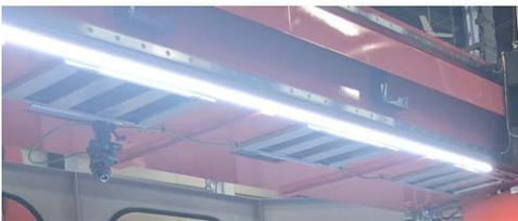
The specially designed, highly rigid tab and slot, structural steel gantry also incorporates a fume extraction
